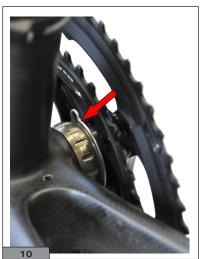
• Move the right crank sideways as if to take it out of the bottom bracket and check the clip is positioned correctly and holds the crank (fig. 11).
