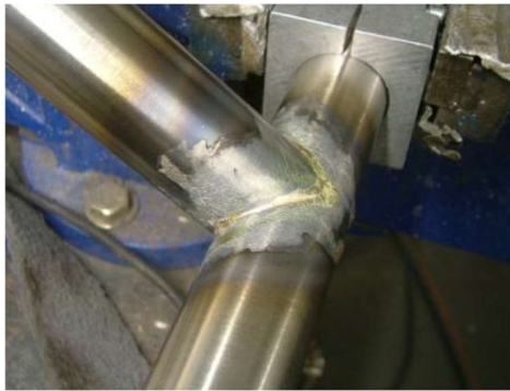
Tacked joint ready for fillet build up
