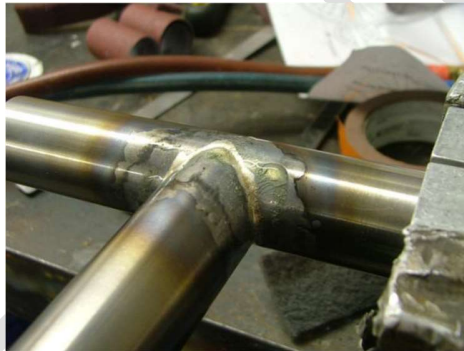
Tubes post brazing and prior to flux removal
