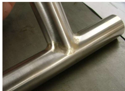
Finished joint after polishing
