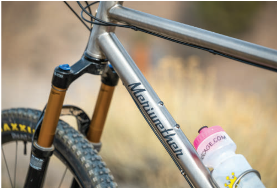
An additional set of downtube bottle bosses adds options when the frame bag is not in use.
