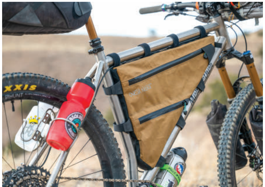
Although the frame's titanium tubeset is thicker and larger in diameter than standard builds, they still look small compared to most carbon and aluminum frames.
