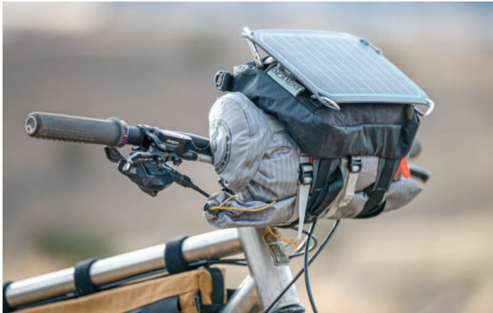
Zach runs a small solar panel on top of his handlebar bag to charge small electronic devices on longer trips.
